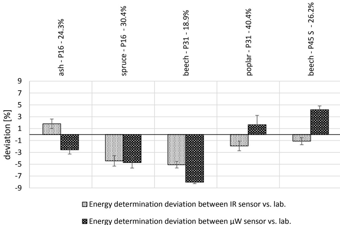
Figure 5 Comparison between the effective energy and that measured via the IR and μW sensors
