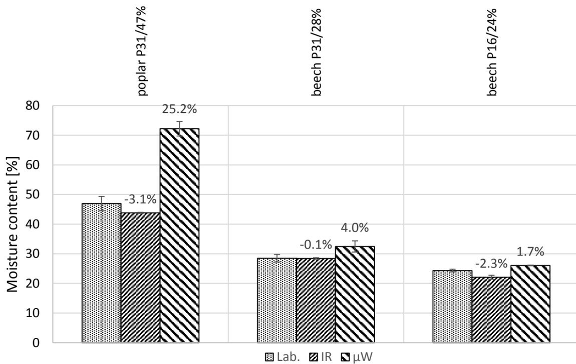
Figure 8 Comparison between the effective humidity and that measured by the IR and  $\mu$ W sensors
