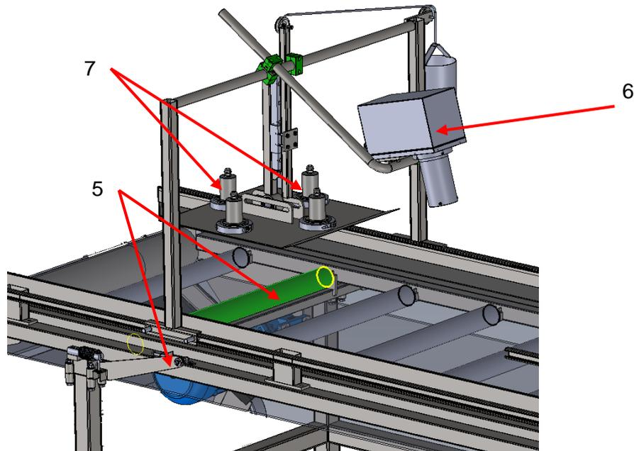
Figure 2 positions of mass and moisture sensors on the measuring conveyor
