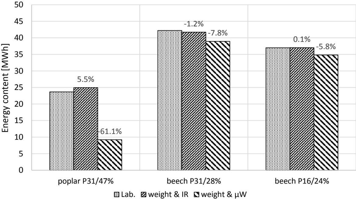
Figure 9 comparison between the effective energy and that determined via the IR and  $\mu W$  sensors
