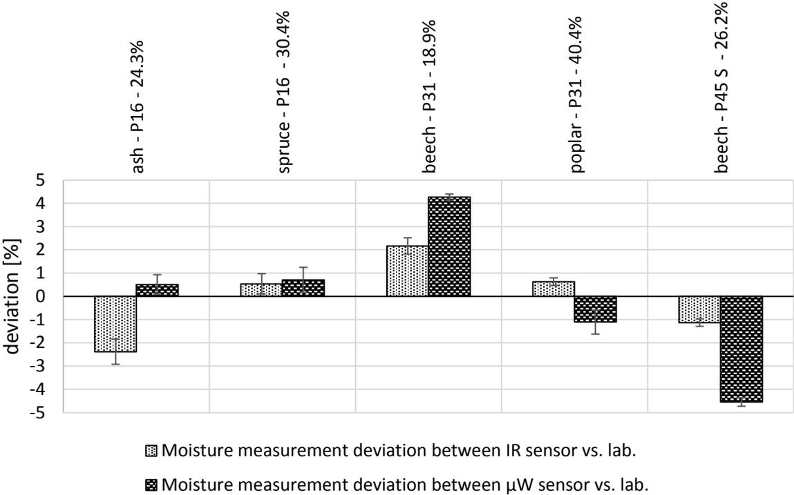
Figure 4 difference between the effective humidity and that measured via the IR and μW sensors
