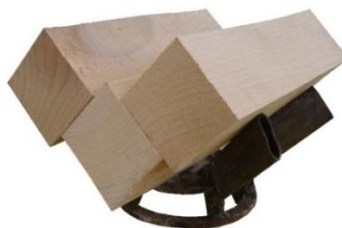
Fig. 7 - Calibrated wood log arrangement on dedicated combustion holder.
