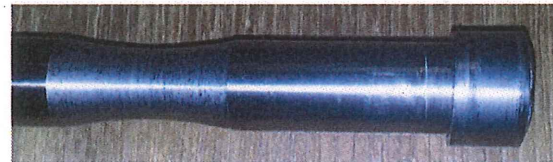
Figure 14. Bush after more than 10000 revolutions.
