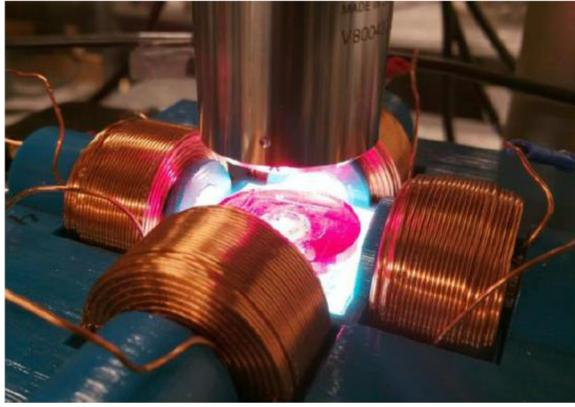
FIG. 4. The experimental set-up: The four electromagnets produce a homogeneous magnetic field in the workspace. The electromagnet consists of a soft-magnetic FeCo core (the diameter is 13.5 mm and the length 30 mm) wound with 0.7 mm diameter copper wire to a total outer diameter of 53.5 mm. For image capture a 20× Mitutoyo objective lens (NA = 0.52) is coupled to a high-speed camera (BASLER acA2000).
